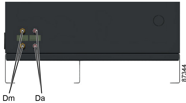
Figure 15: Condensate drain connections, Full-Feature
