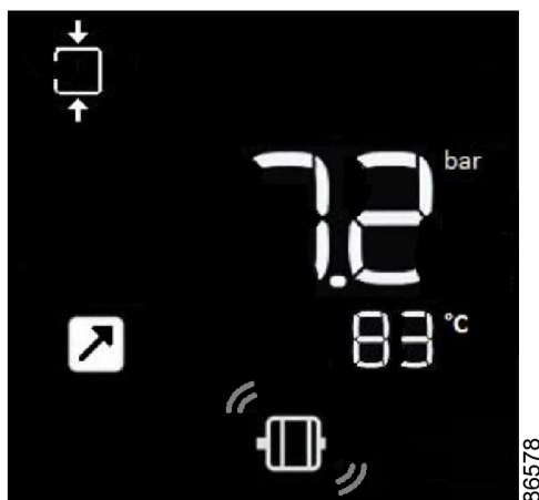
Figure 25: Main screen with shutdown indication, motor overload
