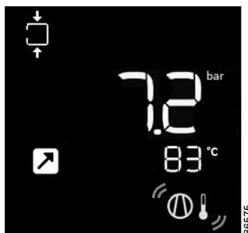
Figure 22: Main screen with temperature switch shutdown
