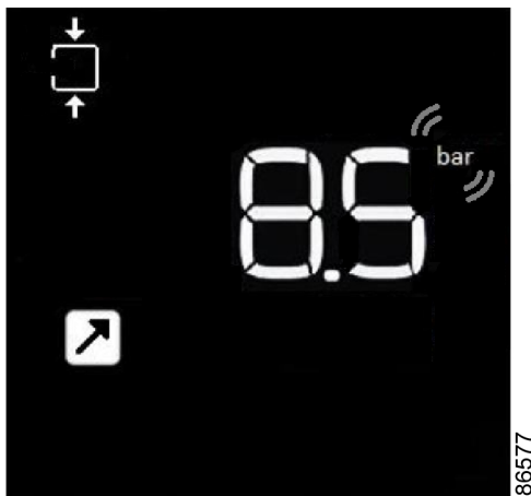
Figure 24: High outlet pressure
