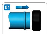
Slide the seal over the edge of the pipe so that it sits flush with the lugged edge.
