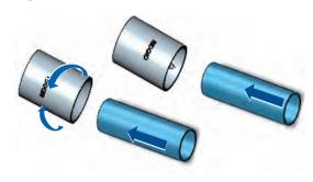
Use a file for DN63-DN200 to chamfer the outer edges; Make sure of a deburring tool to deburr the inside of the pipe end.
