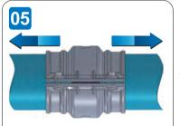
Pull the pipe back towards the outside of the clamshell to complete alignment.
