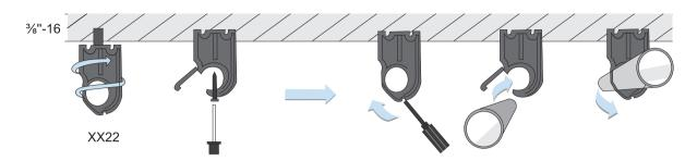
AIRpipe's pipe clips are designed for versatility. They can be secured via all-thread rod through the clips internal %"-16 nut, or mounted directly with wall anchors.
