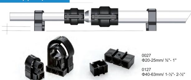
Spacer clip 0027 is used to create a level plane for 3/4" or 1" diameters transitioning to 1-1/2", 2", or 2-1/2". Spacer clip 0127 is used to create a level plane for 1-1/2", 2", or 2-1/2" diameters transitioning to 3" or 4".
