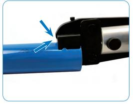
• Release the jaws. Press the trigger and crimp the pipe until a "snap" sound is heard.
