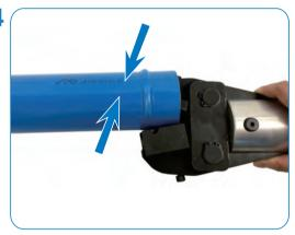
• Renew the operation until the required minimum number of lugs for each diameter is finished.
