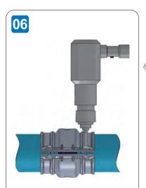
Tighten the pre-fitted screws. Flush the clamshell halves together to complete assembly.
