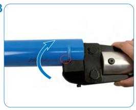
• Re-open the two jaws to remove the pipe and rotate the pipe slightly. Put the jaw side to the mark position.
