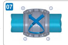
For effective assembly, tighten the screws in an "X" pattern. To disassemble, perform the same operation in reverse order.
