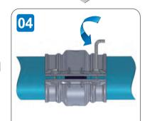
Tighten the pre-fitted screws.
